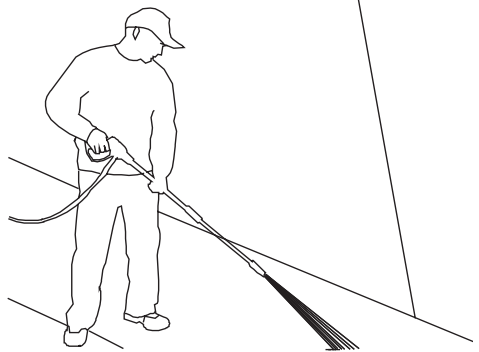
Figure 4- Optimum angle to cleaning surface
