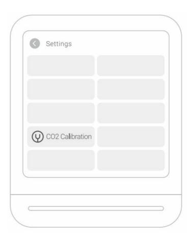
• If the CO2 reading is abnormal, you can go to "O", choose "CO2 Calibration" > "Manual Calibration", then follow the instructions on the device to proceed.
