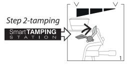
After grinding, pull the lever (A20) down fully (do not remove portafilter). For a perfect result, you can do it twice.
