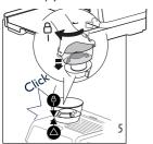
Put the container back inserting it in the coffee mill. The container is correctly inserted when the arrow ▲ is lined up with the 合 symbol and you hear a "click".
