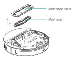
(2) Cut o hairs around the brush with knife, and clean the main brush with the other end of the knife.
