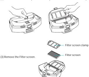
(4) Clean the filter screen and clamp with cleaning brush.
