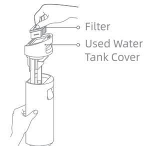
3. Rinse the Used Water Tank and the tank cover with clean water. Clean the tank by the provided cleaning brush.
